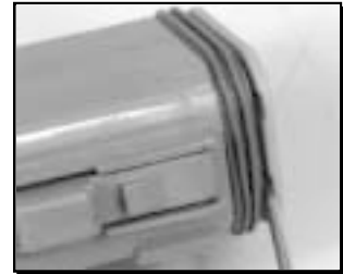
Figure 8 Disassembling the Male Housing.
