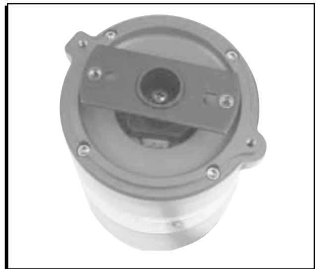
Figure 1 Removing the Original Cap, Rotor and Drive.
