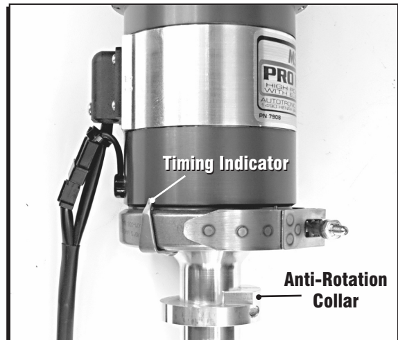
Figure 1 Positioning the Chevrolet Generator.
